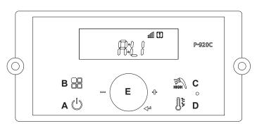
1. STATUS DISPLAY MODE (When button is pressed for 5 seconds When power to display panel is ON , status display will be activated)
