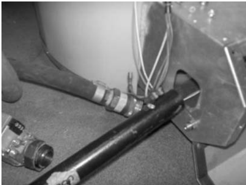
Step 9: Slide manifold out through side flange opening in Burner Box
