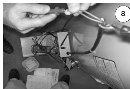
Checking continuity of upper sensor wire harness.
