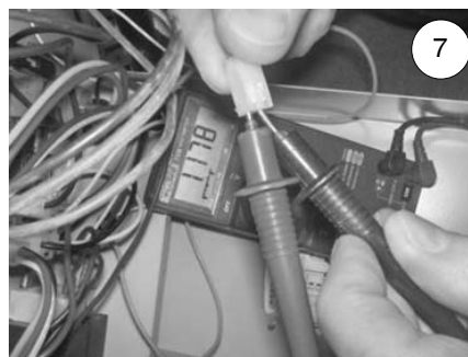
Measuring upper sensor resistance through wire harness (disconnected at control board).
