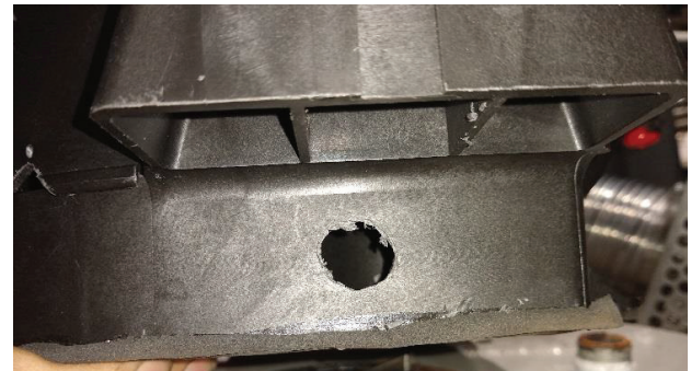
Drill through the exterior molded wall without damaging the interior molded wall at the location shown (right).
