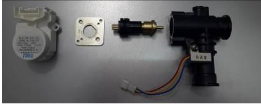
Figure 24 – Inlet Water Valve Composed by a Motor Stepper (left) and a Flow Sensor (right)
