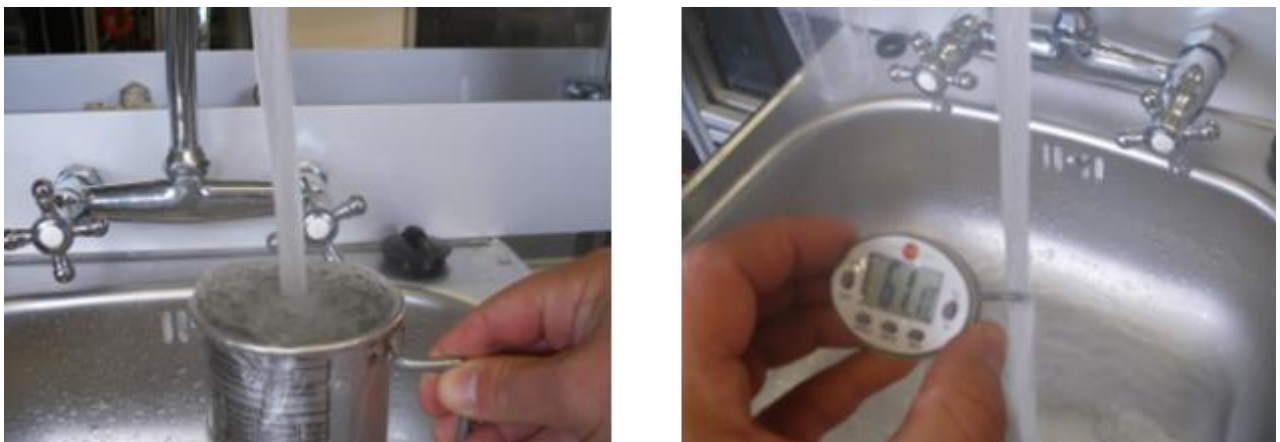
Figure 6 – Use of Water Flow Meter and Thermometer
