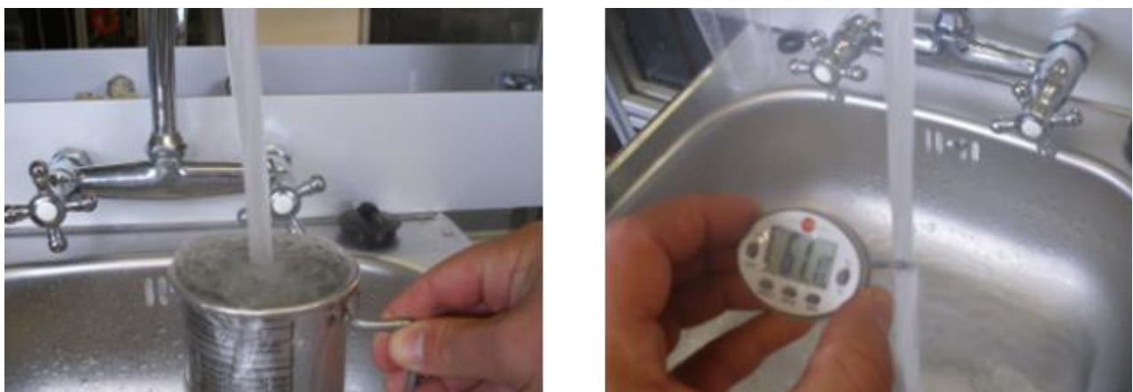
Figure 6 – Use of Water Flow Meter and Thermometer
