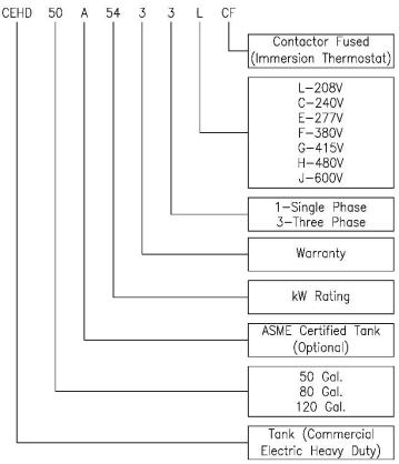
In the field this information is determined from the heaters rating plate located on the front of the water heater.
