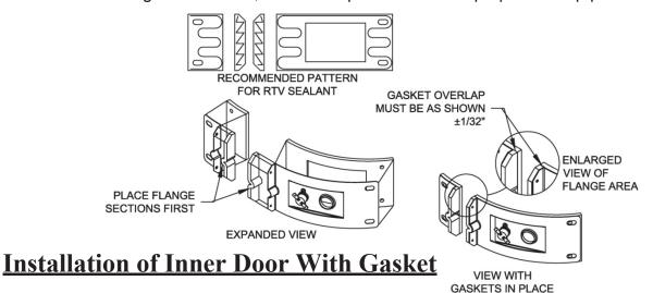
Step 10. Clean any residual gasket residue or other debris from combustion chamber surface before installing the inner door/gasket assembly.
