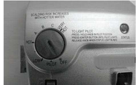
Rotate knob counter-clockwise to the "OFF" position
