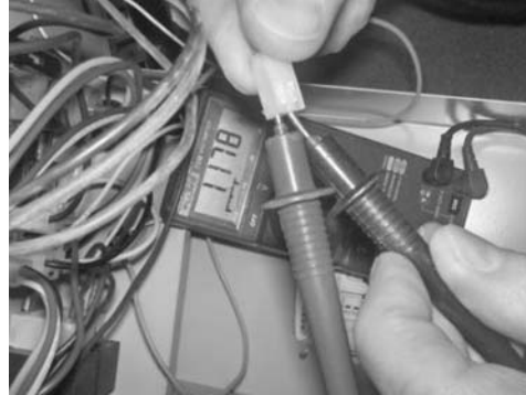
Measuring upper sensor resistance through wire harness (disconnected at control board).
