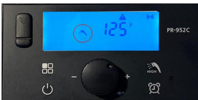
4. Select temperature between 125 to 140°F and press Adjustment Dial to confirm
