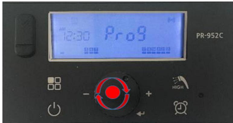
Use the blinking cursor and center dial (turn +press) to select the desired active program times
