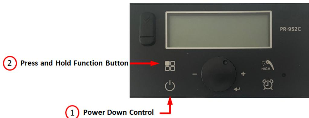
Rotate dial to Parameter 8: RC (DHW Recirculation). Push the center dial and select the type of Recirculation that will be used by rotating the dial. Select the type of Recirc by pushing the center dial
