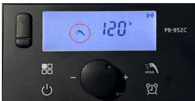
3. Press + Hold the Hot Water Temperature button until 125° F and triangle with exclamation mark appears
