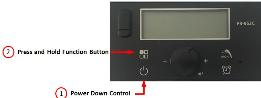
Rotate dial to Parameter 11: RC (DHW Recirculation). Push the center dial and select the type of Recirculation that will be used by rotating the dial. Select the type of Recirc by pushing the center dial
