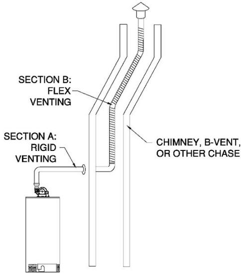
**Note:** Section A refers to equivalent vent length of rigid polypropylene vent, which may include 45° and 90° elbows. Flexible polypropylene venting must be installed in a vertical or nearly vertical orientation. Installations of polypropylene venting must adhere to the vent manufacturer’s installation instructions in order to comply with UL-1738 or ULC-S636.
