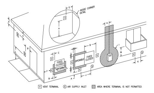
Figure 1 - Vent Terminal Clearances
