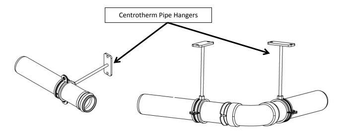
Steel joint connector rings (available from Centrotherm supplier) must be used at each pipe joint. The connector rings ensure that the joints do not separate under heavy loads. These connector rings must be used to comply with ULC-S636 requirements. See following photo with the joint connector attached to the pipe sections.
