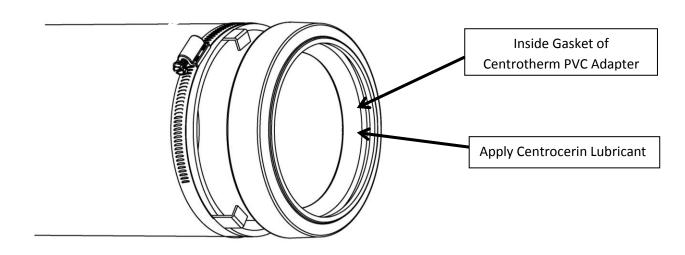
Insert the male end of the straight pipe or elbow into the flanged gasketed end of the PVC adapter. Push the pipe or elbow into the adapter using a twisting motion to fully insert the pipe into the gasket inside the adapter.
