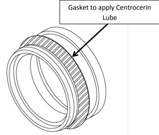
Insert male gasketed end of Centrotherm PVC adapter into PVC pipe coupling.
