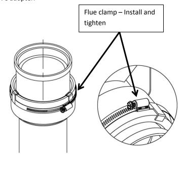
For the exhaust venting for all power vent and power direct vent models, insert the PVC Adapter into the Exhaust Outlet Adapter. On residential models, tighten the clamp to secure the PVC Adapter.
