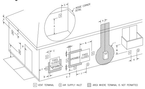
Figure 1 – Direct Vent Terminal Clearances
