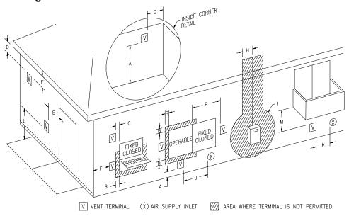
Figure 1 – Direct Vent Terminal Clearances
