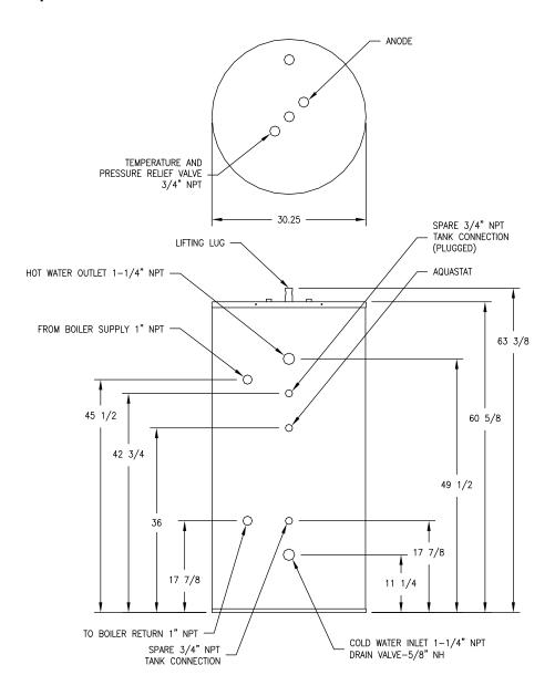
Figure 2 – Tank Layout (120 gallon model)
