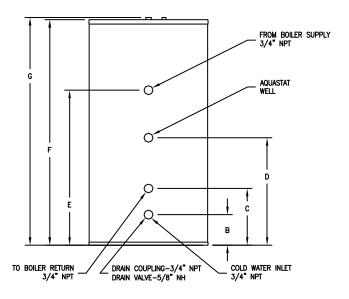
Figure 1 – Heater Layout (40, 52, 75 single exchanger models)
