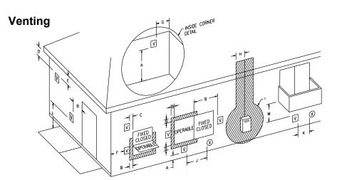
$\boxed{\hspace{0.1in}}$  vent terminal  $\hspace{0.1in}$  ar supply inlet  $\hspace{0.1in}$  area where terminal is not permitted Figure 1 - Vent Terminal Clearances
