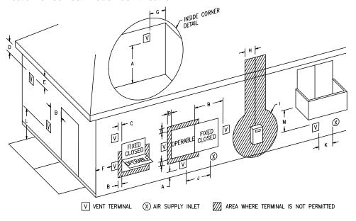
Figure 1 - Vent Terminal Clearances
