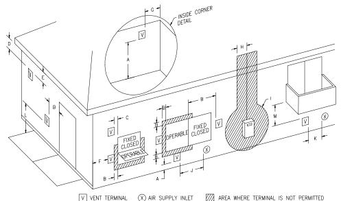
Figure 1 - Vent Terminal Clearances
