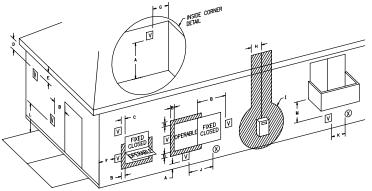
V VENT TERMINAL (X) AIR SUPPLY INLET 🕅 AREA WHERE TERMINAL IS NOT PERMITTED
