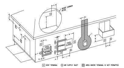
Figure 2 Direct Vent Terminal Clearances
