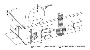
Vent Terminal Clearances (Other than Direct Vent or "Power Vented" Installations)
