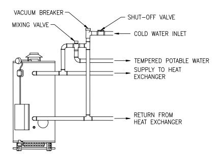
Suggested Piping Arrangement For Side Connections
