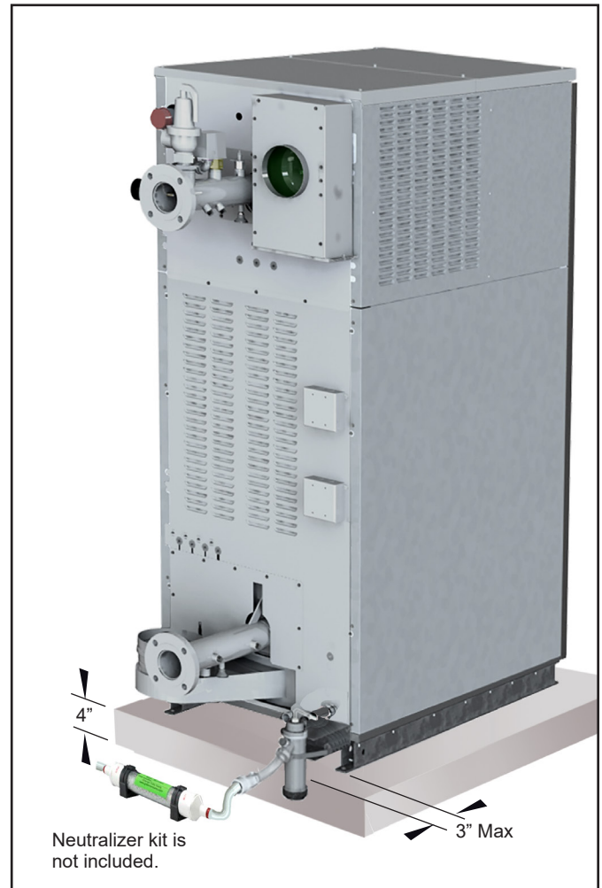
Figure 16. Raised 4" Concrete Platform
