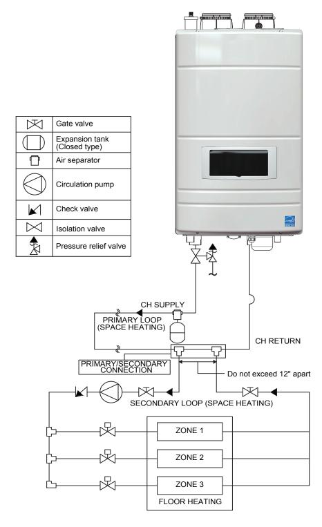
Figure 11. Plumbing Diagram using zones and circulation pumps
