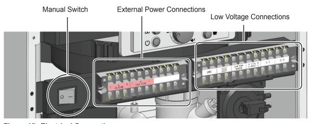
Figure 15. Electrical Connections
