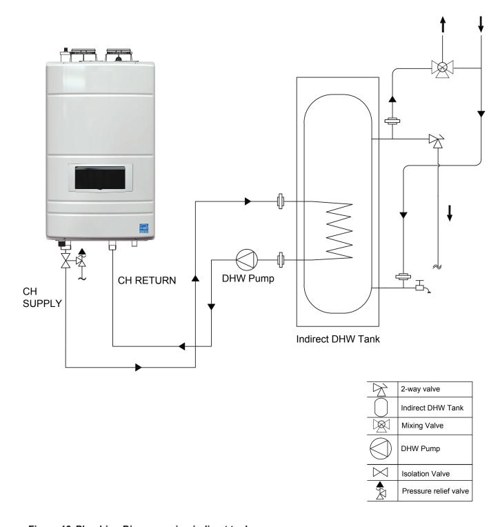
Figure 13. Plumbing Diagram using indirect tank
