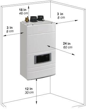
Figure 3. Locating the Appliance. Minimum clearances to Combustibles.
