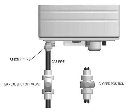
Figure 9. Gas Line Valve Detail
