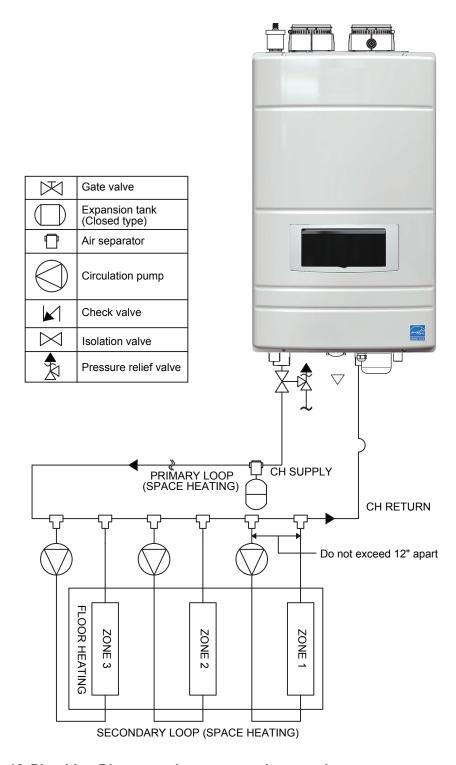
Figure 12. Plumbing Diagram using zones and zone valves
