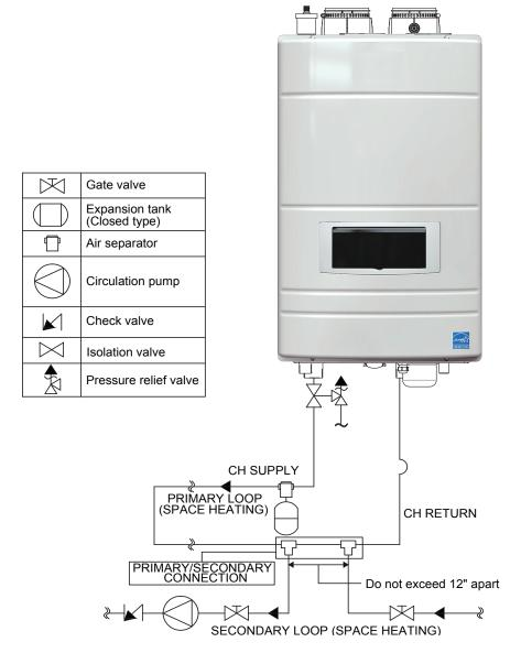
Figure 10. Plumbing Diagram using a Diaphragm Type Expansion Tank
