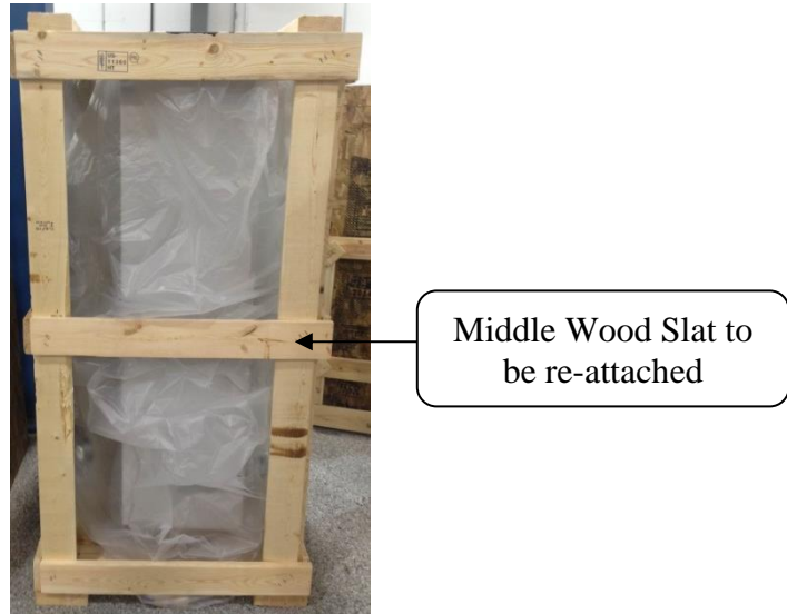
Fig. 21 Water Heater Shown in Crating
