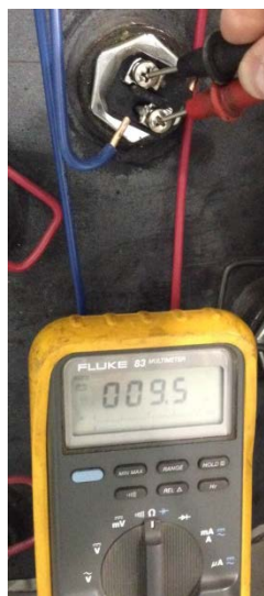
Figure 14. Resistance Check of Element using a Multi-Meter
