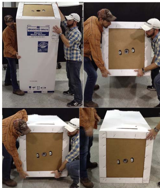
Figure 2: Place the water heater on its side as shown with two people.
