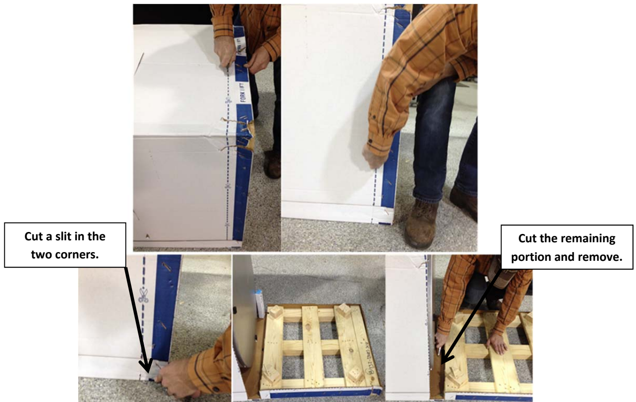
Figure 3: Cut the carton along the dotted line, cut 2 slits in the bottom, and cut the remaining portion.
