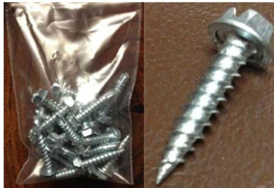
Figure 4: Self tapping screws used to attach the legs to the water heater.
